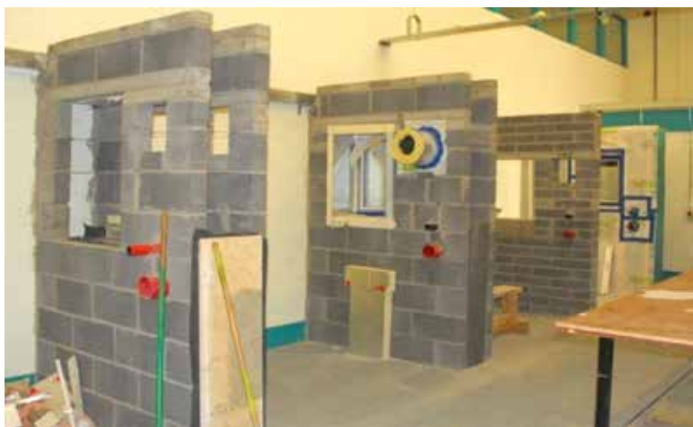
Figure 88: Selection of practice models fixed against a wall, including windows and service penetrations. © MosArt
