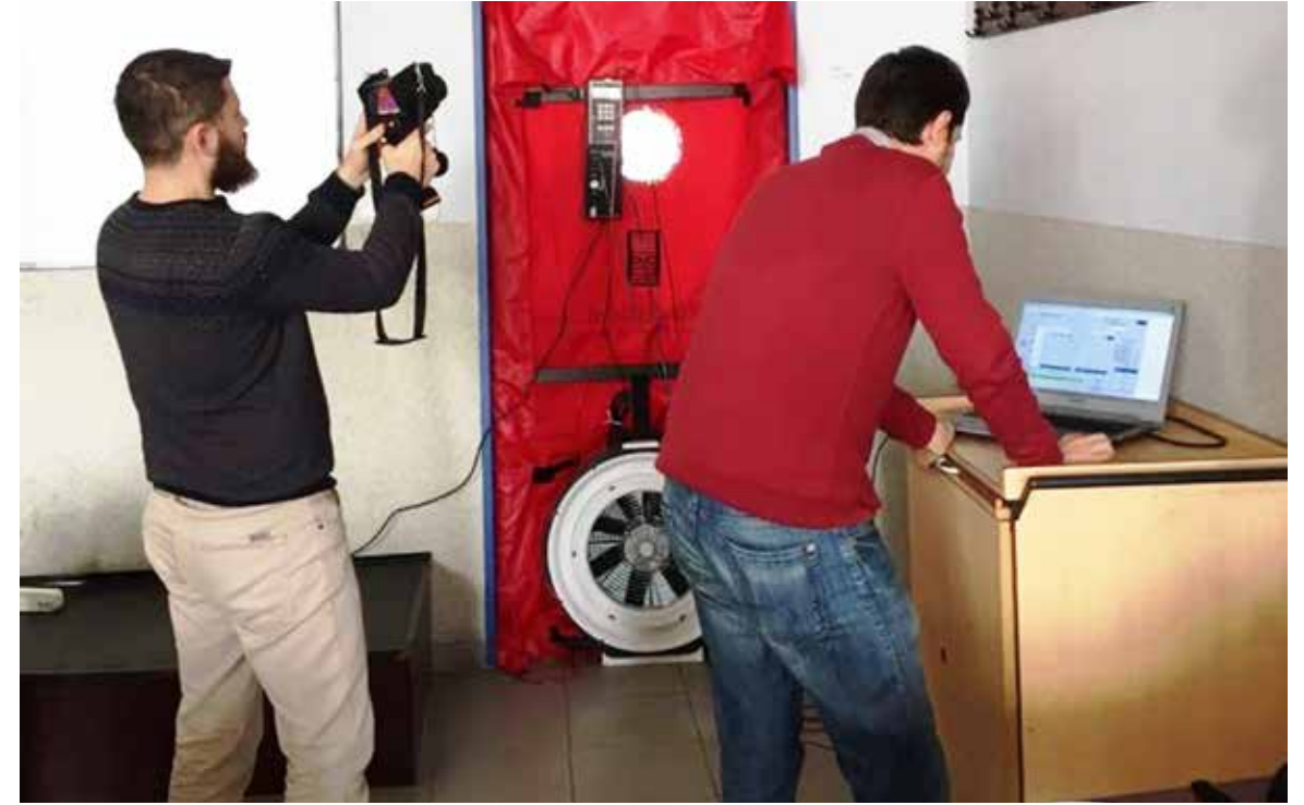
Figure 60: Demonstration of Blower-Door Test Units. © EGE
